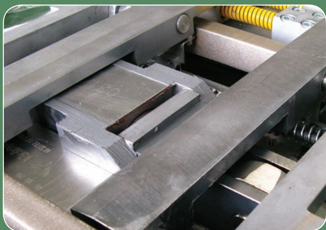
Trailing mechanism is integrated within the lock body
